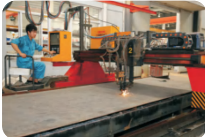
数控高速火焰切割机 Digital-controlled fire cutting machine from USA
