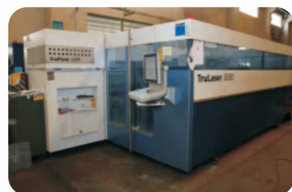
德产数控激光切割机 Digital-controlled laser cutting machine from Germany
